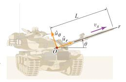
$$v_s^2 = 2\ddot{r}(2L - 0) \quad \Rightarrow \quad \ddot{r} = v_s^2/(2L). \tag{2}$$
